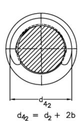
$$\begin{array}{lll} b & = 2.55 \\ d1 & = 20 \\ d2 & = 18.1 \\ d3 & = 17.55 \\ d4 & = 22.65 \\ d4 & 2 & = 23.2 \\ Description = H & 20,0 \\ FN & kN & = 4.70 \\ \end{array}$$
